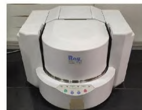
Figure 1. The equipment used for the study: 1. Optical microscope Keyence VHX-100; 2. X-ray fluorescence spectrometer Shimadzu EDX-720. Photos M. Stamberova
